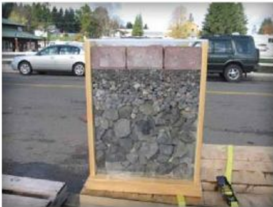
Figure 3. PICP cross section utilized ICPI recommendations on stone sizes for bedding, base and subbase.
